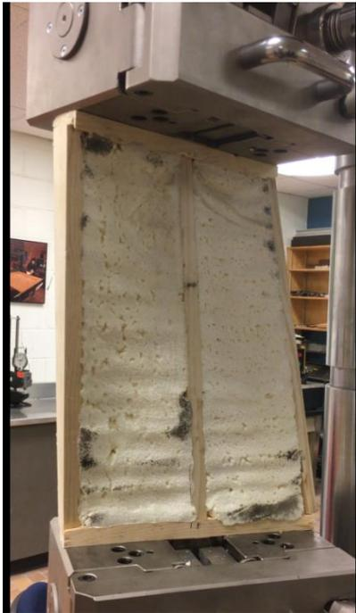
Looking at Table 1 we can see that the section that withstood the highest stress was a three-stud empty section. Ultimately an outside stud buckled on this section after the plates had failed, but it was one of only three sections that did not have any significant knots on its studs. It may be interesting to note that each section with knots present in the studs always failed on or around the knot, as can be seen in Figure 11 below.
