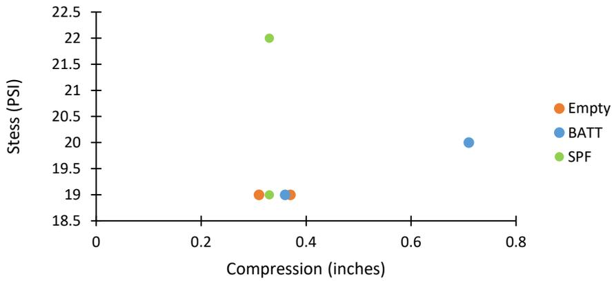
In addition to the direct comparison of maximum stress, it is interesting to see the full graphical representation of each test throughout their entire durations. While the ADMET Expert Hydraulic Testing System automatically creates a Stress/Position graph, it is unable to overlay past test results. Therefore, to generate a graph of combined full test results the raw data was extracted for each test and
