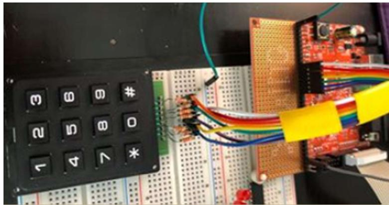
Figure 42: Laser Harp Keypad Set-up
