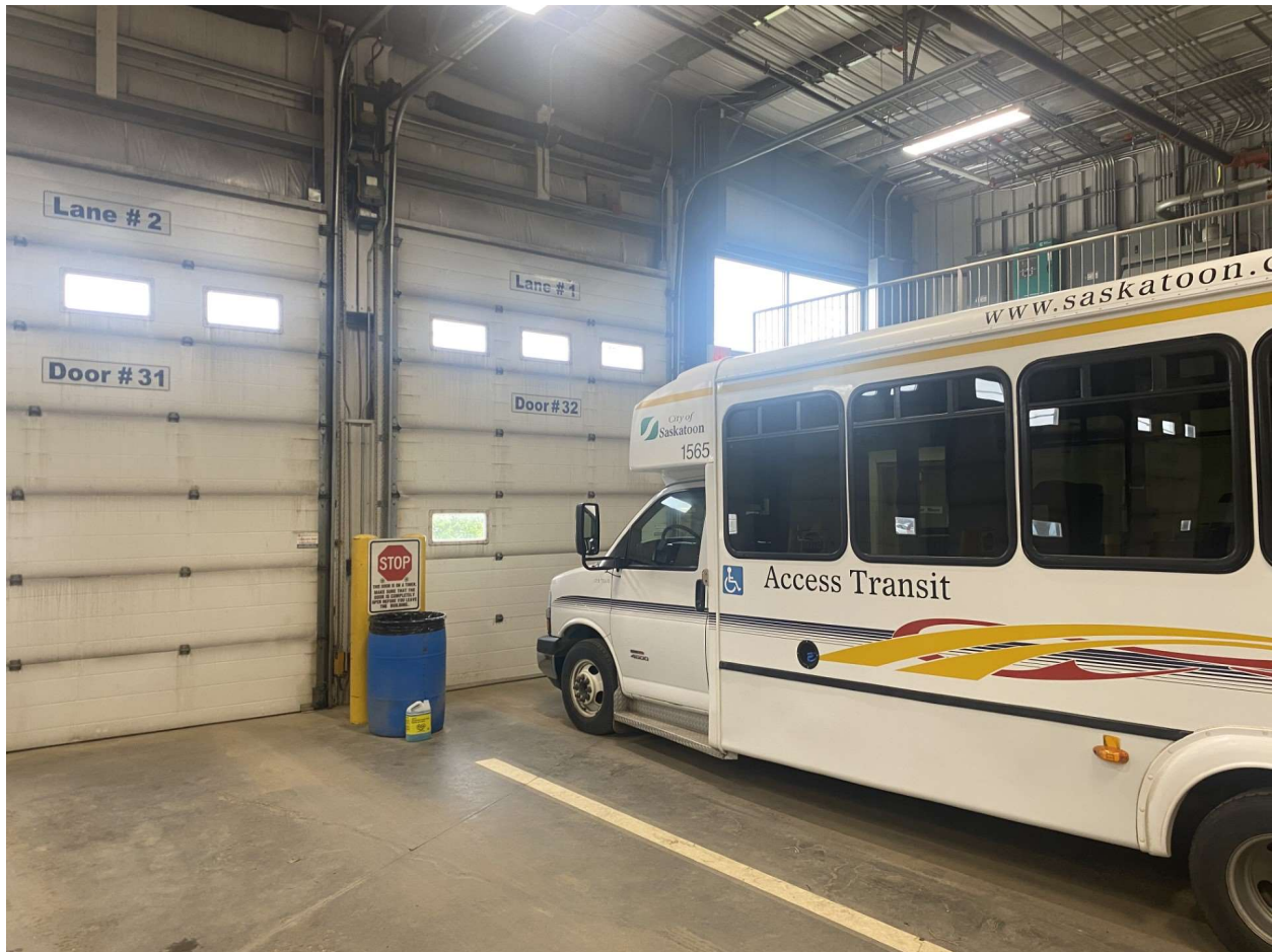
Fig. 18. An 11-foot tall Access Transit Bus by a 14-foot tall door
