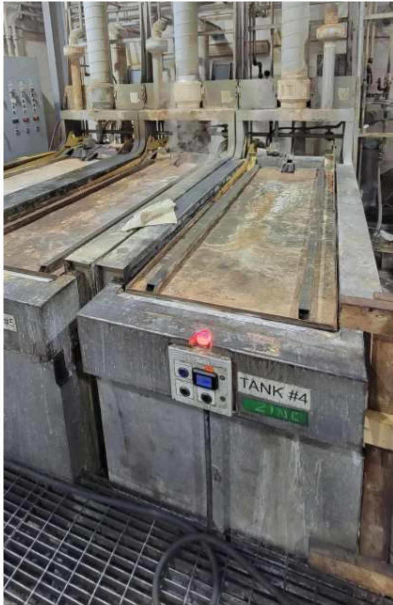
Figure 2. Photo of Current Phosphate Dip Tank Set-up in Argus
